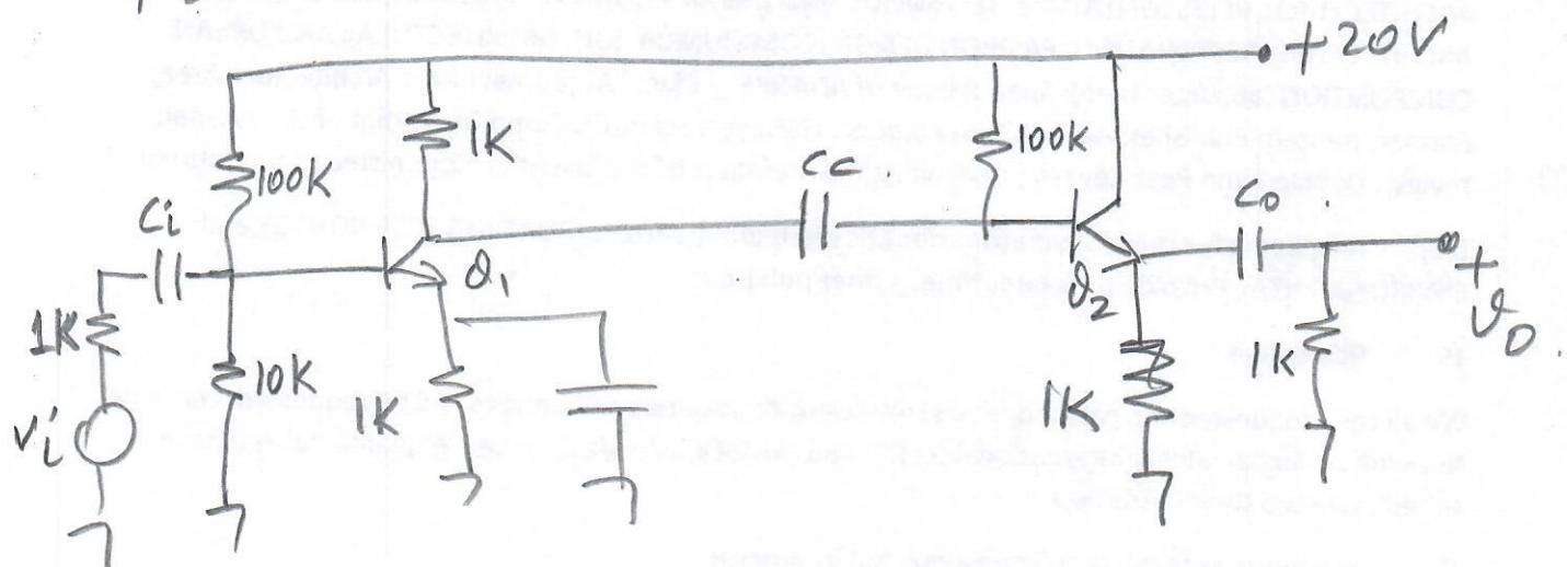
$h_{fe} = 100$ ,  $V_0 = 0.6V$ ,  $I_{CO} = 0A$ ,  $V_{CESAT} \approx 0V$ .
