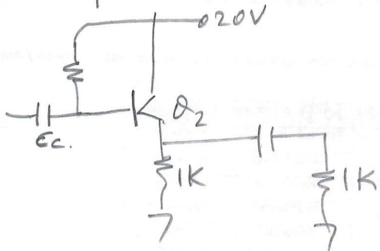
DC Analysis / DC equivalent circuit:
