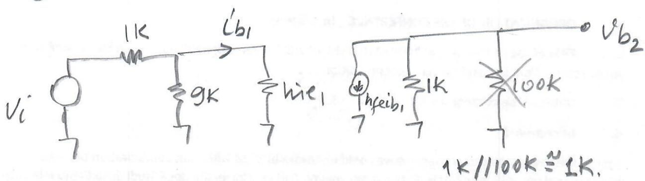
$$h_{ie2} = 260 = \frac{h_{fe} \cdot 26 \text{ mV}}{I_E \cdot R} , \quad h_{ie1} = 1,9 \text{ k} \text{ (calculated)}$$
