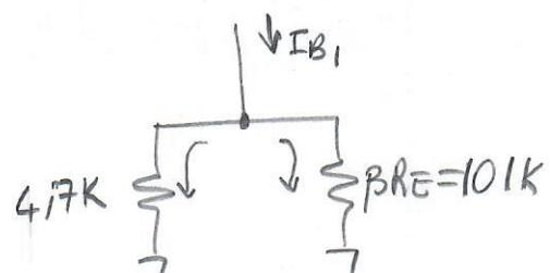
$$I_{E1} \approx \frac{V_{E1}}{R_E} = \frac{V_{B1} - V_{BE}}{R_E} = \frac{4.95 - 0.7}{1k} = 4.25 \text{ mA}$$
