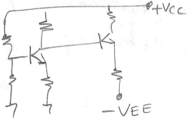
$$I_{EQ_{\text{new}}} = \frac{V_{EE_{\text{old}}} - V_{EE}}{R_E}$$
