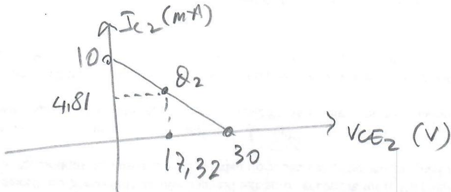
$$V_{C_2\bar{Q}} = V_0 = 30 - 2K I_{C2}$$
