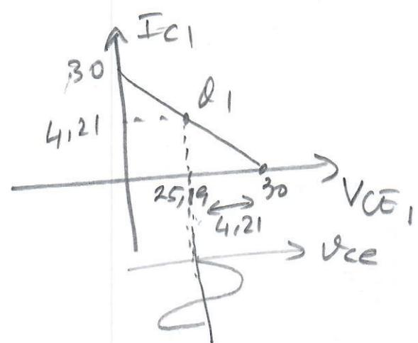
$$\text{So, } V_{C\bar{E}_1} = V_{CC} - 1K I_{C1} \\ = 30 - 1K \cdot I_{C1}$$
