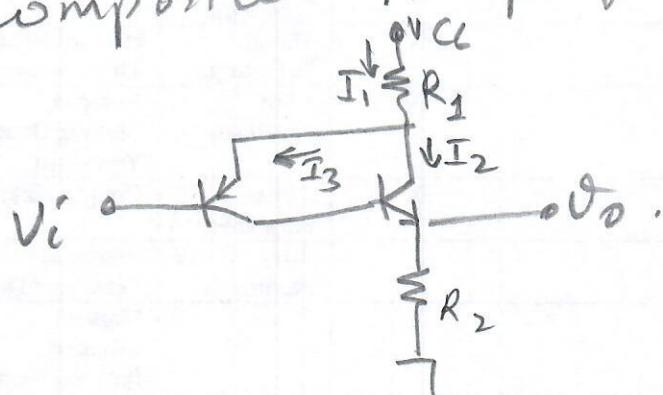
$$V_{CC} = I_1 R_1 + V_{EB} + V_i$$
